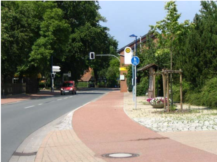
Fig. 22 Common pedestrian and cycling path in Germany. Source: Planungsgemeinschaft Verkehr (PGV) and German Road Safety Council (DVR).
