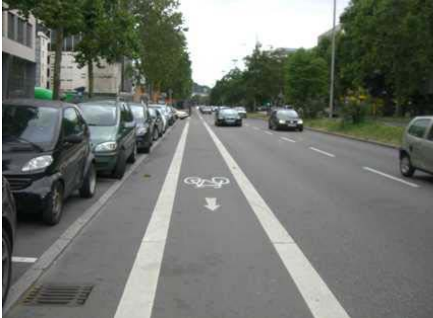
Fig. 18 Cycle lane with protection space from the doors of cars which are parked adjacent to the lane. Source: Planungsgemeinschaft Verkehr (PGV) and German Road Safety Council (DVR).
