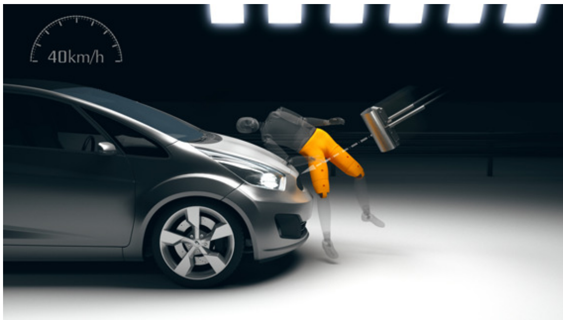
Euro NCAP's upper leg impact test
