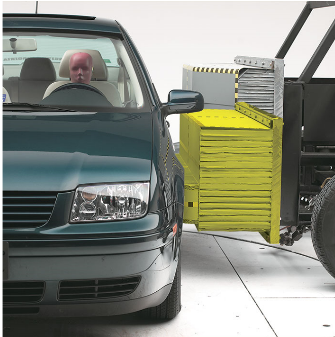
Insurance Institute for Highway Safety (IIHS), United States – Side crash test with side barrier representing an SUV
