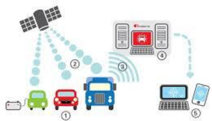
The Cobis Telematics solution in the vehicle (1), obtains vehicle trip data and also GPS position (2), which are transmitted via GSM/GPRS/3G (3), to the server at the Cobis Service Centre (4), from where they are made available to the customer via phone or internet (5).
