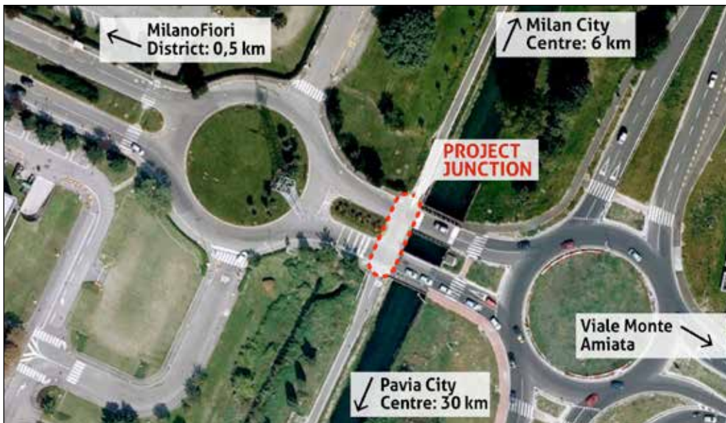
picture 05 Aerial photo of the selected project area at the Alzaia Naviglio Pavese junction. Here the Strada Alzaia Naviglio Pavese bike path was interrupted and safety conditions for crossing the road were missing.
