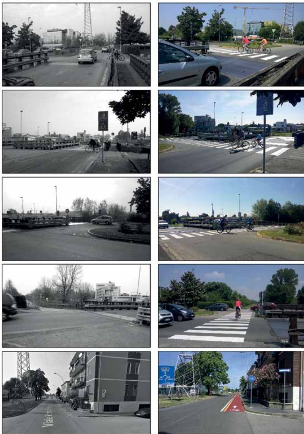
picture 16 Photos of the previous and current situation at the project junction. On the left, the situation before the realization of the infrastructural intervention, on the right it is possible to see how the junction changed after the realization of the proposed safety measures (zebra crossing, vertical road signs, flashing lights). At the bottom the previous and current situation in viale Monte Amiata, regarding the realization of the new bike lane.
