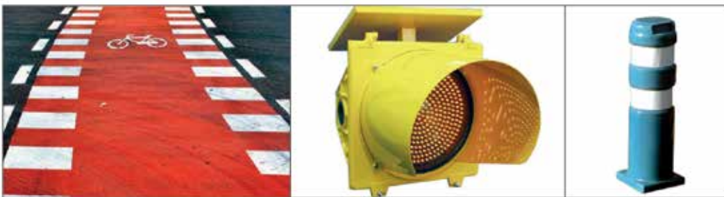
picture 08 Some of the proposed safety devices for the Alzaia Naviglio Pavese project: - red painting for highlighting the passage of bikes; - flashing lights for making visible the intersection between the road and the cycle path; - road posts for avoiding U-turns of cars.
