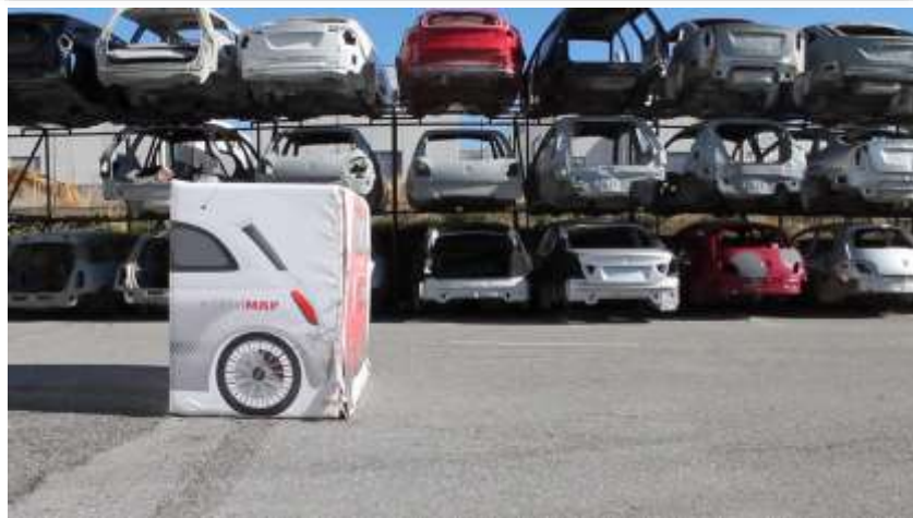
Urban AEB (LIDAR sensor)
