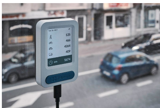
The Telraam S2 device counting the number of road users per category. This device will, in the near future, also be able to more precisely differentiate between types of road users, with the heavy vehicles category for example being further differentiated into vans, trucks, buses, trailers and tractors.
